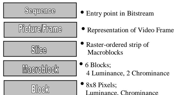
Figure 1. AVS Layered Data Structure
