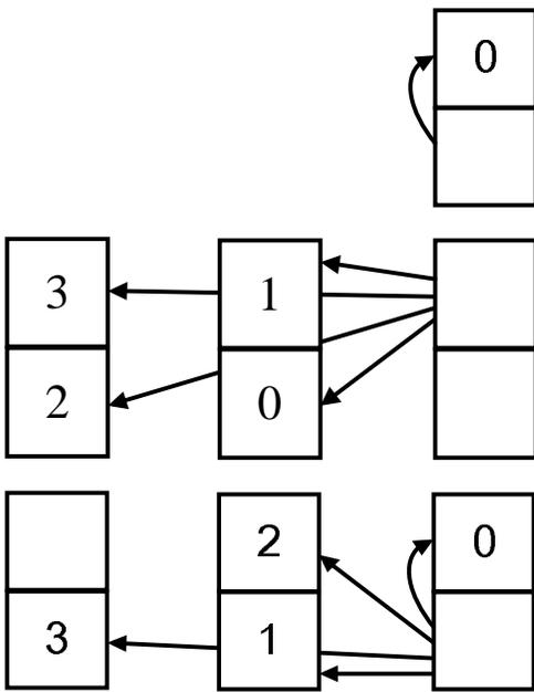
Figure 7. Interlaced P-Frame Prediction.
