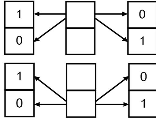
Figure 9. Interlaced B-Frame Prediction.
